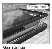
The piston rods should be wiped with a clean dry grease-free cloth or piece of clean kitchen towel. Gas springs should be operated monthly and should be replaced when the pressure drops.
