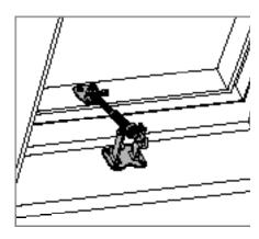
Re-attach the spindle (Part 3) to the ironmongery supporting bracket (Part 2) and spring clip (Part 1). Test the ironmongery is operating.
