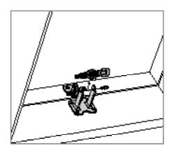
Detach the inner spindle (Part 3a) from the spring clip (Part 1) by pulling back the plunger. Remove the spindle from the ironmongery support bracket (Part 2) by unscrewing the retaining screws (Part 4).
