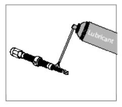
Fully unwind the spindle (Part 3). Apply a water-displacing spray (such as WD 40) to the spindle. Fully wind the spindle out to ensure all of the thread is lubricated.
